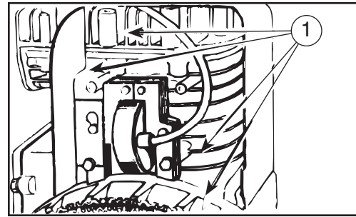
FIGURE D.3 - CLEAN COOLING SYSTEM
